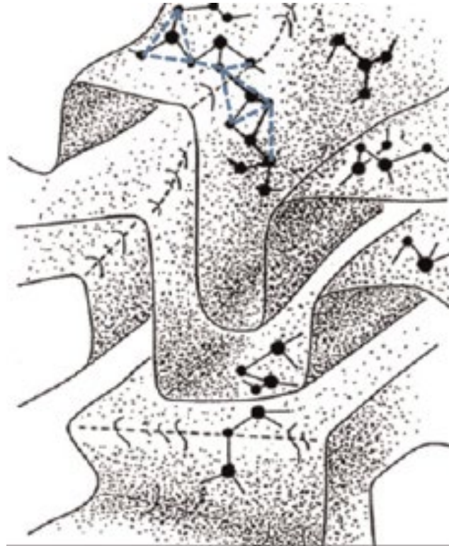
AsS(Se) 3 glass. The three- and the two-fold coordinated circles represent As and S(Se) atoms, which form AsS(Se) 3 trigonal pyramids (dashed lines), which produce corner- and edge-shared connections and extend to distorted layer-like clusters.
